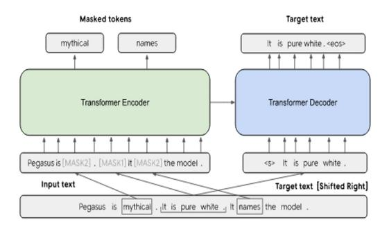
PEGASUS' fundamental architecture is a Transformer encoder-decoder.
